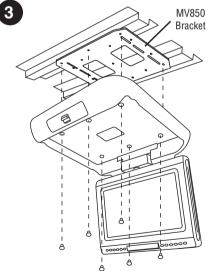
Attach the screen housing to the metal support bracket using the screws removed in Step 1.
